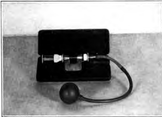
Fig. 37. Adjustable whistle for determining the frequency of the highest audible sound.
